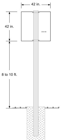
The length of your posts is determined by the configuration of your scoreboard display, its height above the ground, and the depth of your footings. Footing size is also related to the cabinet height and configuration. To some degree, the depth of the footings will be determined by the equipment available to the installer. In general, a smaller diameter hole needs to go deeper than a larger diameter hole. The trick is to create footings hefty enough to provide stability for the sign structure.
