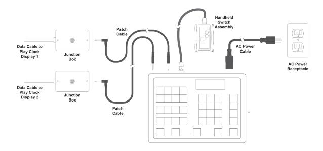
If your play clock package includes a ScoreLink RF Communications system, the power receptacle may be the only consideration on the control console side of the installation process. For details about ScoreLink, consult the documentation that ships with the product. Otherwise use the stereo patch cables to plug the console into the junction boxes.
